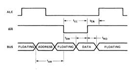
Input and Output Waveforms for A.C. Tests
